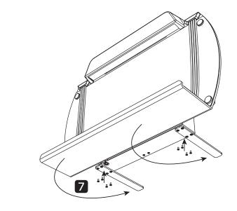
7. Unscrew 8 screws at the bottom and tune the support pieces backward. Install 8 screws back finally.
