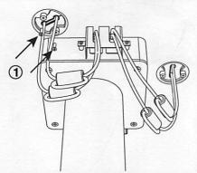
1) Detached the cable clip by unscrewing the 2 screws.
