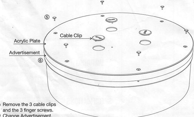
(5) Remove the 3 cable clips
