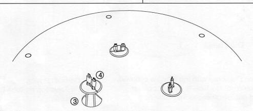
3 Remove cables from cable clip.
