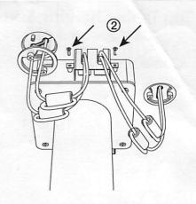
2 Unscrew the 2 screws on cable cover.
